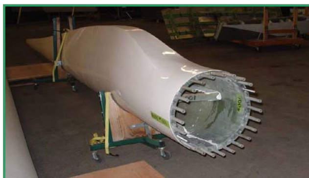
Figure 26. Root End of BSDS Prototype Blade Showing Flatbacks and Embedded Anchor Rods
