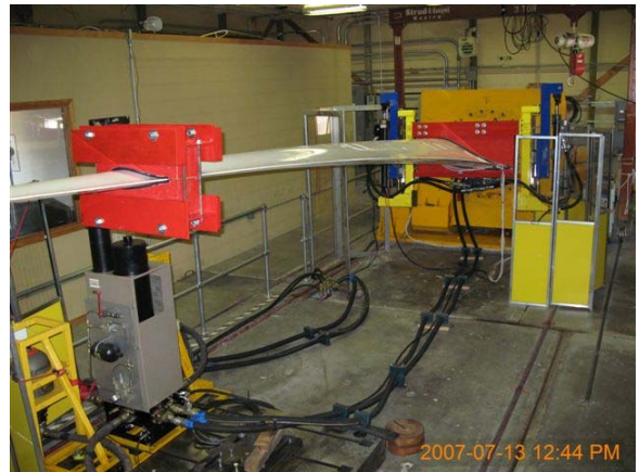
Figure 30. TX-100 Fatigue Test at NREL's NWTC Facility
