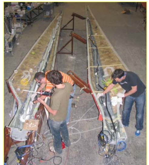
Figure 24. Installation of Sensors During SBlade I Fabrication
